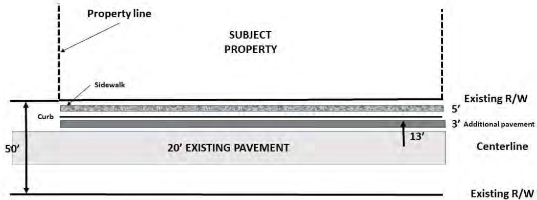
REQUIRED PAVEMENT OF SUBSTANDARD CITY STREET (URBAN CROSS SECTION) (FROM SUBSTANDARD 20 FOOT WIDE PAVEMENT TO 26 FOOT WIDE STANDARD WITH CURB AND GUTTER AND SIDEWALK ALONG FRONTAGE)
