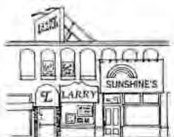
These signs block building elements and create a chaotic image
